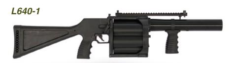
**L640-** - A spring-advance magazine drum launcher, with a six-shot capacity and rifled barrel. Features include: Double-action trigger, lock push button and chamber out-of-line safeties, 40mm, 1:47 twist-rifled 12-inch barrel, combination weaver rail with ghost ring and bead sight, overall length of 23 inches/584mm with stock collapsed and 34 inches/864mm extended or fixed, unloaded weight of 11.3 lbs/5.2 kg, utilizes 40mm x 158mm max length munitions.
